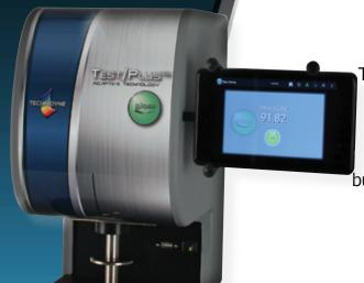
The Technidyne TEST/Plus™ Gloss combines industry standardized measurement technology with an innovative control package that allows the user to tailor build their testing and evaluation capabilities. This new addition to the TEST/Plus™ product line is built to meet your Gloss testing needs;
